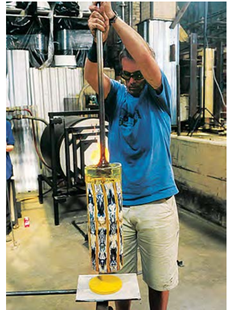
...and attached to the rolled-up tile to close the cylinder.
