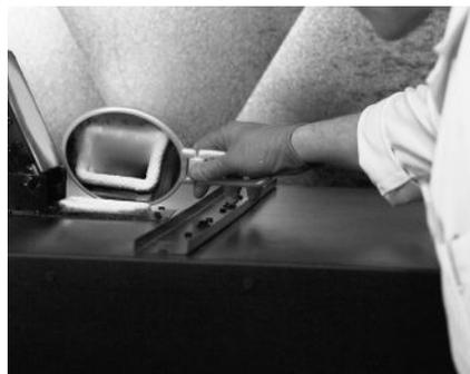
Figure 7: using a mirror to check for condensation.
