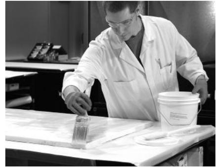
Figure 8: Brushing qf-180 onto the fiberboard shelf.
