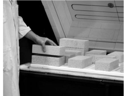
Figure 11: weighting the fiberboard shelf with bricks.
