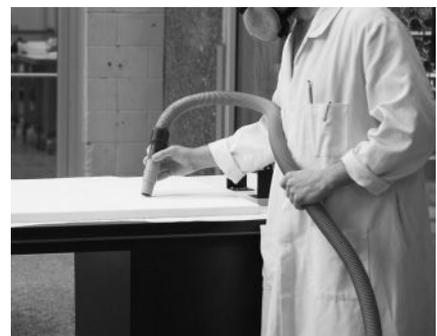
Figure 10: vacuuming dust from the shelf after sanding.
