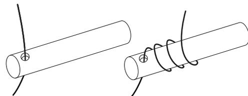
**PIPES:** You can make stringers in the shape of spring-like coils using a 1” (2.5 cm) diameter steel pipe. These coils can then be carefully cut into sections that will form perfect circles when kilnformed. The pipe illustrated here is 15” (38 cm) long with 0.5” (1 cm) holes drilled through the wall about 1” (2.5 cm) from the pipe’s end. Pull the glass stream through the drilled holes. As the glass flows, twirl it around the pipe and then cut or break it at the end of the pipe.
