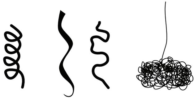
**HAND PULLING:** Many types of lines require only handwork (while wearing Zetex or Kevlar gloves). If the glass is viscous enough you can pull it at intervals to create stringers of fluctuating thickness. At these low temperatures the glass can also be pulled into curves. At very high temperatures when the stream is extremely thin and fast moving you can make delicate bird’s-nest shapes by allowing the stream to freefall.
