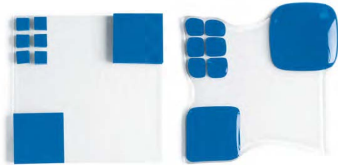
Figure 4; Stacking glass unevenly and close to edges can result in distortion of the shape of the fired glass.
