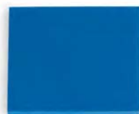
Figure 3: One, 1/8" (3 mm) layer fired to 1500°F (816°C). Notice how the edges pull in.
