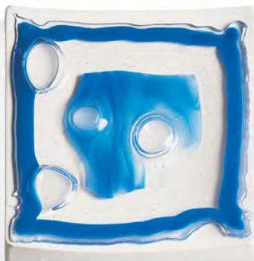
Figure 8: This plate (shown still on the mold) was formed with a single firing for both fusing and slumping. This shortcut caused edge distortion and bubbles.
