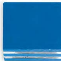
Figure 2: Five, 1/8" (3 mm) layers fired to 1500°F (816°C). Notice substantial spread in area.
