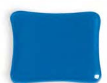
Figure 3: One, 1/8" (3 mm) layer fired to 1500°F (816°C). Notice how the edges pull in.
