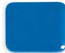
Figure 1: Two, 1/8" (3 mm) layers fired to 1500°F (816°C). Notice that the area covered stays the same and the edges are straight.
