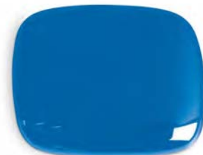
Figure 2: Five, 1/8" (3 mm) layers fired to 1500°F (816°C). Notice substantial spread in area.
