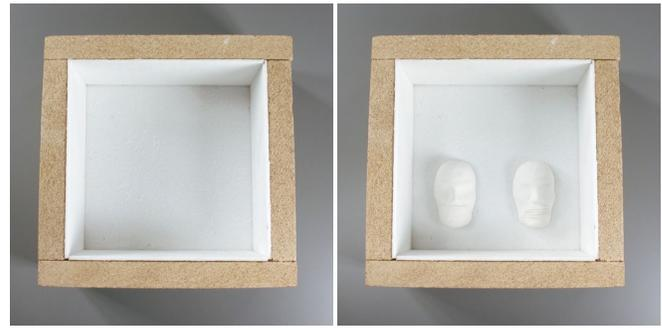
Hydrate the plaster/silica design elements by soaking them in water until the bubbles quit rising (5-10 minutes). This helps to keep the plaster/silica bed from sucking in around the design elements due to differences in humidity. Arrange design elements on the interior base of the box. Check once again to make certain that your work surface is flat and level.
