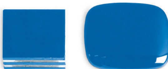
Figure 2: Five 3 mm ( \frac{1}{8} ") layers fired to 1500°F (816°C). Notice substantial spread in area.
