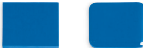
Figure 1: Two 3 mm ( \frac{1}{8} ") layers fired to 1500°F (816°C). Notice that the area covered stays the same and the edges are straight.
