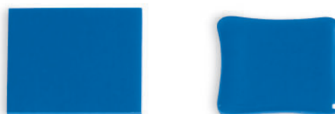
Figure 3: One 3 mm ( \frac{1}{8} ") layer fired to 1500°F (816°C). Notice how the edges pull in.
