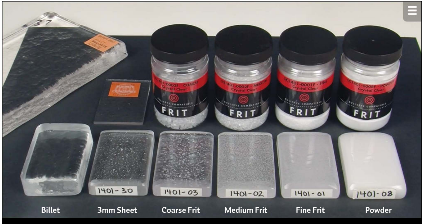
Above: These cast samples were all made from different forms of 1401 Crystal Clear Transparent.
