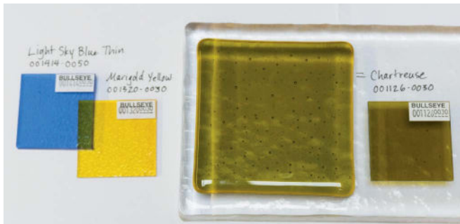
TOP: Light Sky Blue Thin 001414-0050 BASE: Marigold Yellow 001320-0030. Tile shown elevated on a Clear billet for light transmission.
