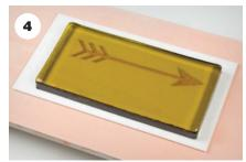
Arrange the fiber paper on a primed kilnshelf. Clean the billet and load it on the fiber paper. Fire with the schedule below.
