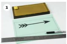
Plan a design based on the billet dimensions, approximately 10" × 5" × 0.75" (127 × 254 × 19 mm).
