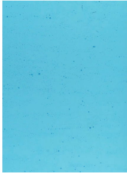
Same, capped with Tekta Clear & fired with schedule provided. Very small bubbles.
