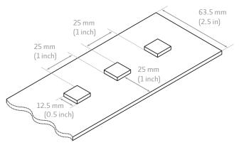
Figure 1: The chip test layup.
