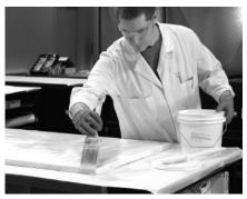
Figure 8: Brushing qf-180 onto the fiberoard shelf.
