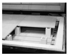
Figure 4: positioning the mullite subshelf units.
