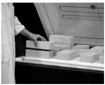
Figure 11: weighting the fiberboard shelf with bricks.
