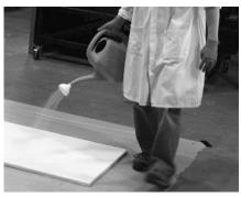
Figure 6: a watering can with a showerhead spout will control the flow of colloidal silica.
