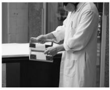
Figure 9: sanding the shelf using a large sanding block.
