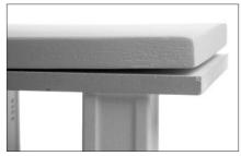
Figure 12: example of a bowed fiberboard shelf corner.
