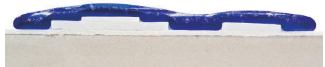
Figure 5: Cross-sectional view of kilnformed glass, fired at 1490°F (~810°C).
