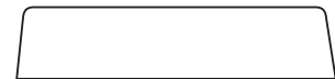
Figure 13: Fiber paper thickness too great. Dams not vertical—finished block won't sit vertically.
