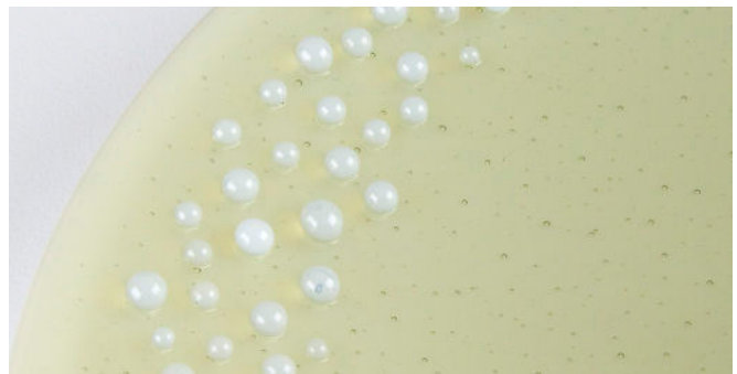
Frit balls made with Opaline Striker coarse frit (000403-0003). (Top and middle) Tack fused together, then slumped. (Bottom) Tack fused to a fully fused plate, then slumped.
