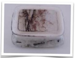
To apply ZYP, work in a well ventilated area or outside, and hold the well-shaken can 10 to 12 inches from the base mold. Hold both the mold and the spray can upright. Apply the first coat using a three to four-second burst of spray in a sweeping pattern across all the mold's cavities. Do not saturate the surface. If it is the first time ZYP has been applied to the mold, it is necessary to apply a second coat of the product.
