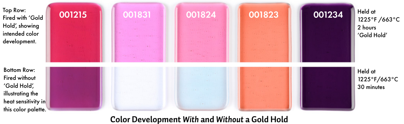
ABOVE: Fired samples of select gold-bearing glasses—Light Pink (001215), Ruby Pink Tint (001831), Ruby Red Tint (001824), Burnt Scarlet Tint (001823), and Violet (001234). Results may vary. For a complete list of styles that require a 'Gold Hold' see page 4.
